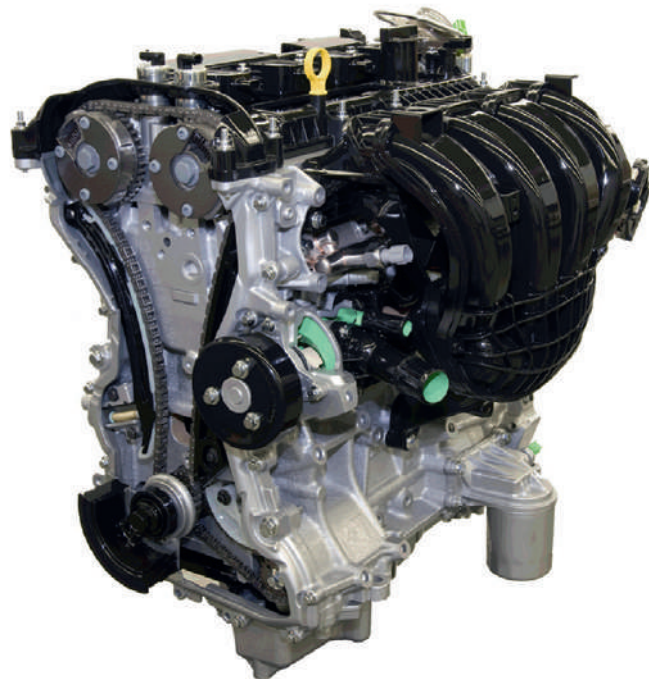
Figure 2.112 Cam drive chain in position on the 2012 Focus engine. (Source: Ford Media)
